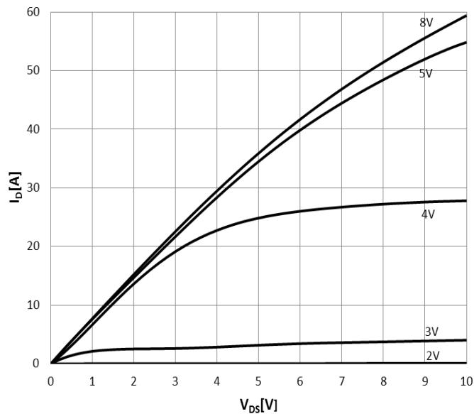
**Figure 1. Typical Output Characteristics  $T_j=25^\circ\text{C}$**
