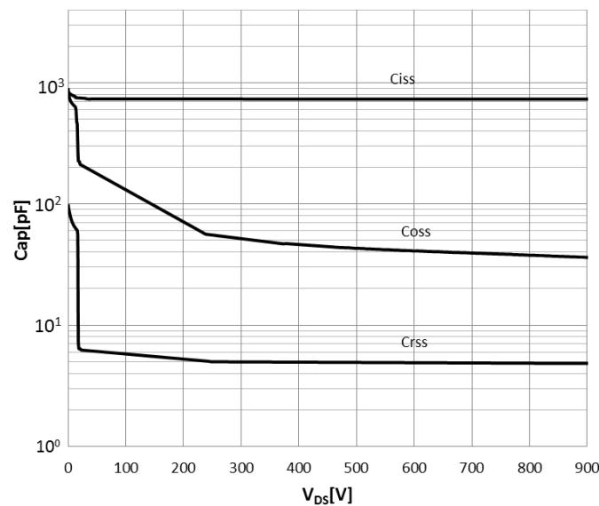
**Figure 5. Typical Capacitance**
