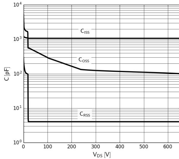
**Figure 5. Typical Capacitance**
