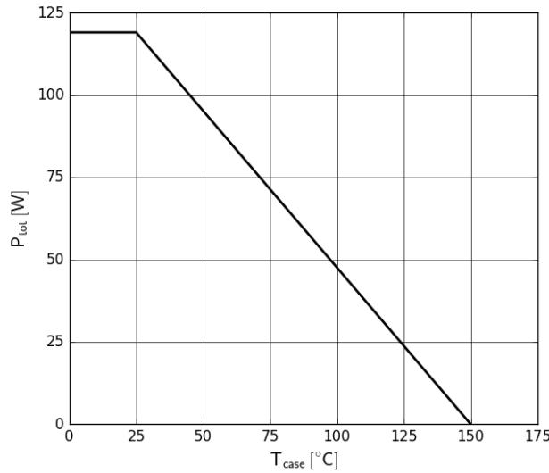
**Figure 9. Power Dissipation**
