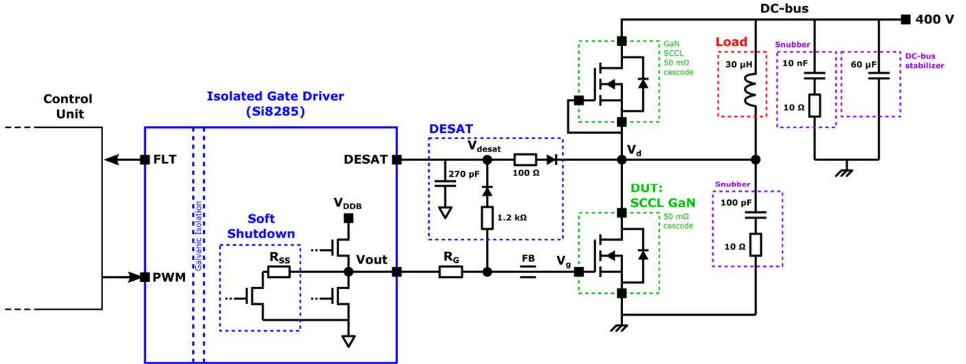
Fig. 6 Short-circuit protection circuitry using GaN power devices with Short-Circuit Current Limiter (SCCL) and a commercial gate-driver with DESAT detection and soft shutdown. An RC network is inserted between the drain and the DESAT terminal to ensure good noise immunity.
