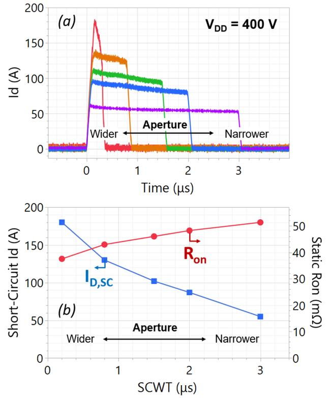
Fig. 5 (a) Short-circuit withstanding time with a DC bus of 400 V and a fully-on gate-bias of 12 V on SCCL devices with multiple aperture sizes. (b) SCWT, short-circuit current and static  $R_{on}$  as a function of aperture size. Smaller aperture yields lower saturation current and longer SCWT, with only limited increase in  $R_{on}$  penalty.
