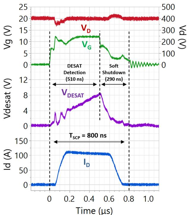
Fig. 7 Short-circuit protection of a SCCL device tuned for a SCWT of 1.5  $\mu\text{s}$  paired with a gate driver with DESAT detection. Thanks to DESAT and soft shutdown, the short-circuit is detected and shutdown in 800 ns, a period sufficiently short to ensure the survival of the SCCL power device with ample margin. The GaN power device with SCCL technology successfully survived the short-circuit event for all 100 repetitions.
