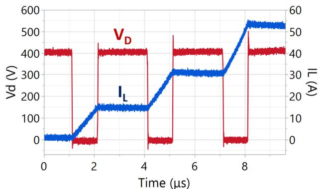
Fig. 8 Successful inductive switching of a SCCL GaN device with a gate driver with DESAT circuitry. With an  $R_g$  of 30  $\Omega$ , we measured a  $dv/dt$  of  $\sim 35 \text{ V/ns}$  in both turn-on and turn-off transients. With an  $R_g$  of 10  $\Omega$ , we recorded a maximum  $dv/dt$  of more than 100 V/ns during turn-off. The short-circuit protection is triggered during switching transients, indicating good noise immunity.
