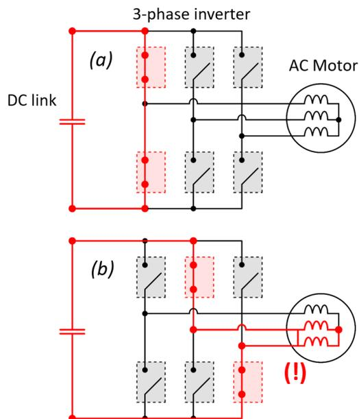
Fig. 1 Power devices in a 3-phase motor drive, showing two short-circuit scenarios: (a) shoot-through between high-side and low-side and (b) short-circuit across the inductive load.
