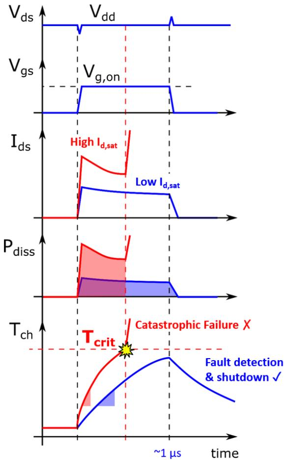
Fig. 2 Schematic waveforms during short-circuit condition for (a) a device with high current and power density leading to steep temperature rise and catastrophic failure before the protection circuitry could intervene and (b) a device with lower current and lower power density, allowing the protection circuitry to detect the fault and safely turn-off the device before the critical temperature to failure is reached.
