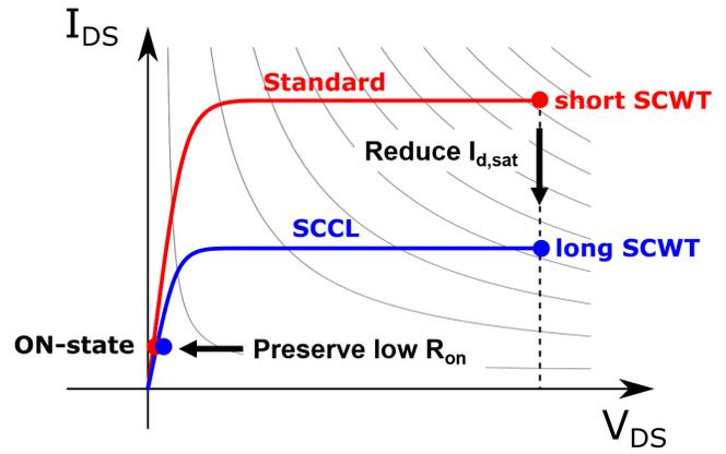
Fig. 3 The patented Short-Circuit Current Limiter (SCCL) reduces the drain-source saturation-current to increase the SCWT while preserving low on-state resistance. Dissipated power contour lines are shown in the background. During short-circuit events, lower saturation-current yields lower dissipated power and longer withstanding time.
