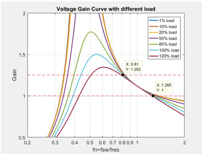
Figure 7. Voltage Gain versus frequency with different load
