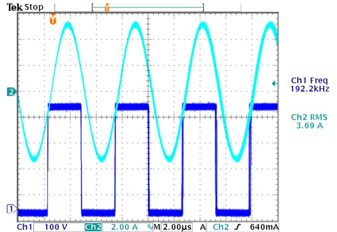
Figure 12. Voltage and current waveform at 600W load
