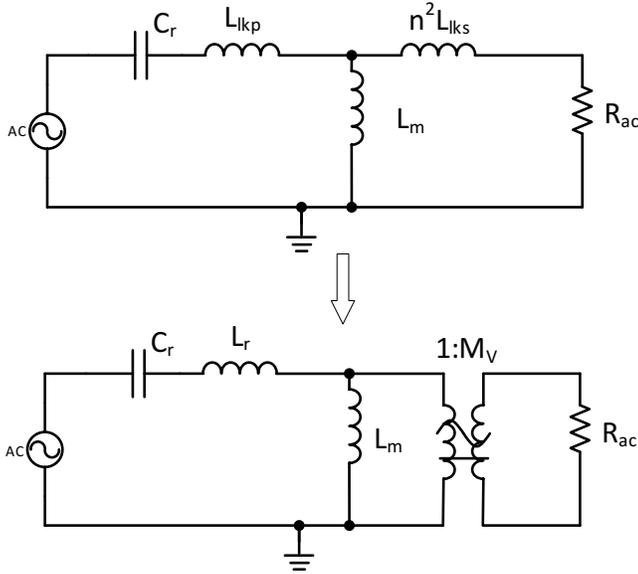
**Figure 4. AC Equivalent Circuit referred to primary side**
