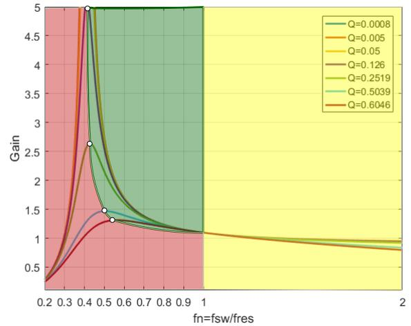
**Figure 5. Gain curve versus frequency ( $L_n=5$ ).
