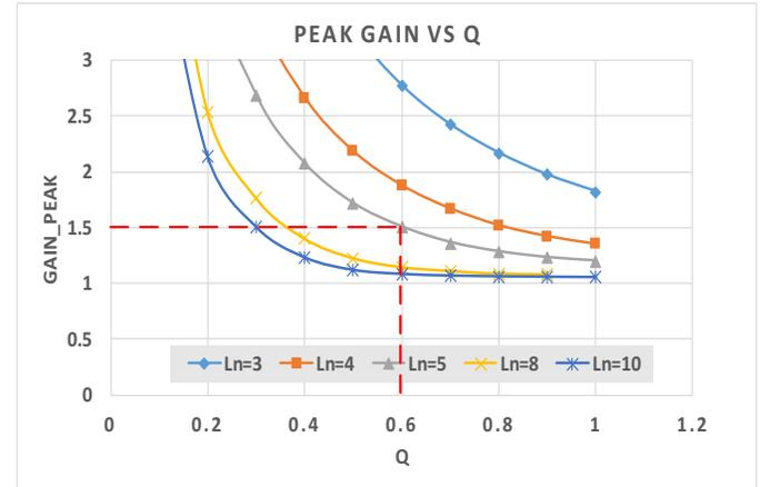
**Figure 6. Peak Gain versus Q for different  $L_n$  [?]**
